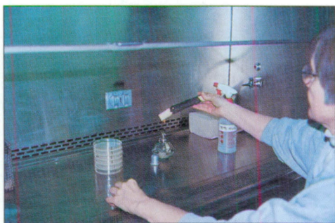
Figure 8. Spraying with 95% alcohol and flaming sterilizes the surface.
